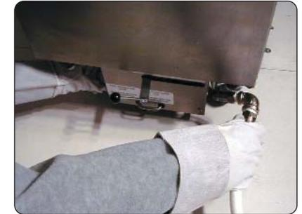
**9.** After rinsing debris, close drain valve and disconnect hose. Push black knob on valve to the right (Oil to Fryer). Turn on pump and refill fryer.
