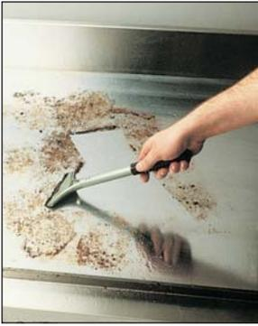
Scrape the griddle with the Keating scraper with replaceable blades.
