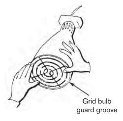
Set bulb guard into groove on shade. (It may be necessary to squeeze shade slightly.)
