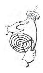
3. Using pliers again, straighten slightly same end of grid until it holds firmly in place.
