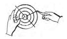
With grid bulb guard in hand take end of grid and bend approximately 45° with pliers.
