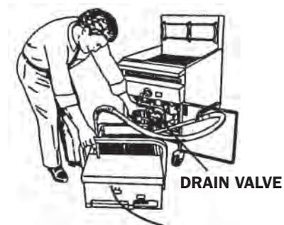
3. Open fryer cabinet door and position portable filter vessel under fryer drain valve. Slowly open drain valve to avoid splashing and permit oil in fryer vessel to drain into filter vessel (Figure 2-1).
