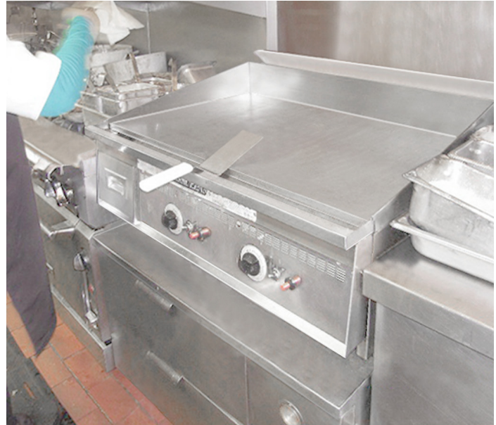
Keating 36x30 Miraclelean gas griddle shown above at Clyde's in Rockville, MD.
