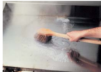
Step 2 - Wash Wash with water and a Keating palmetto brush.
