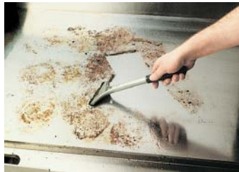
Step 1 - Scrape Scrape the griddle with the Keating scraper.
